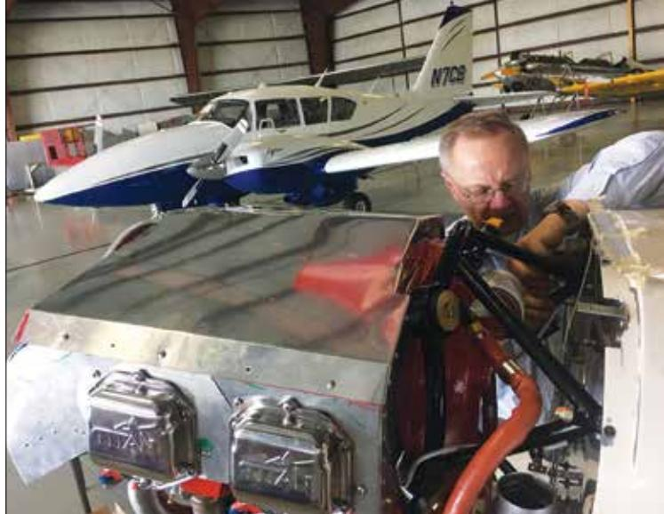
(Left) Making progress on the baffles. Important notes were written with a Sharpie. (Right) The completed baffles. An aluminum top was added to form a plenum. That's Bob Siegfried installing components on the firewall.
