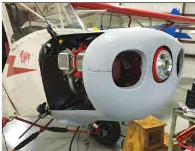
(Left) Painter’s tape was used to accurately mark the cowling door before cutting. (Right) With the new nose bowl installed, the cowling is close to being completed.
