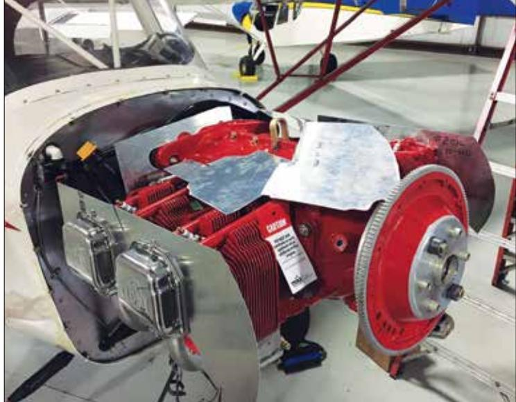
(Left) After stripping the firewall of all components from the Jabiru installation, the new oil cooler for the Titan engine was installed. (Right) Without documentation, figuring out the baffles was a bit of a puzzle.
