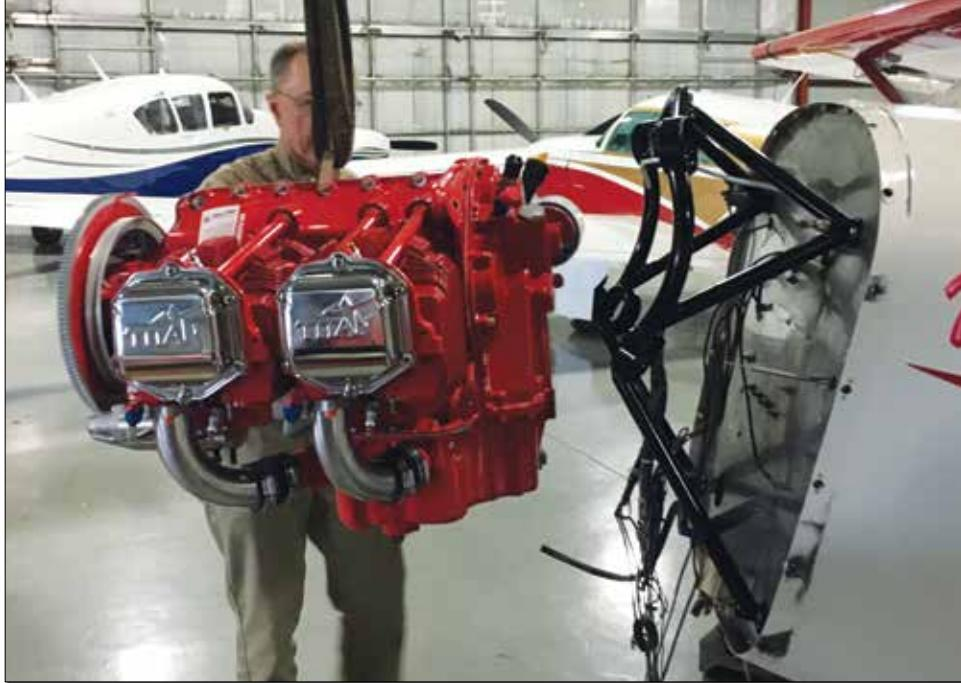
Although they were pretty sure it would work, before the installation in *Ziggy*, Legend had never actually mated a Titan engine to a Cub with a Jabiru firewall and boot cowl.
