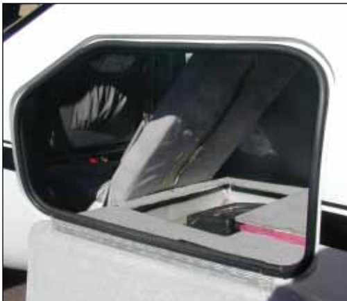
The GlaStar's baggage compartment has a small third seat installed and under-floor storage. The certified version doesn't include those modifications as options.
