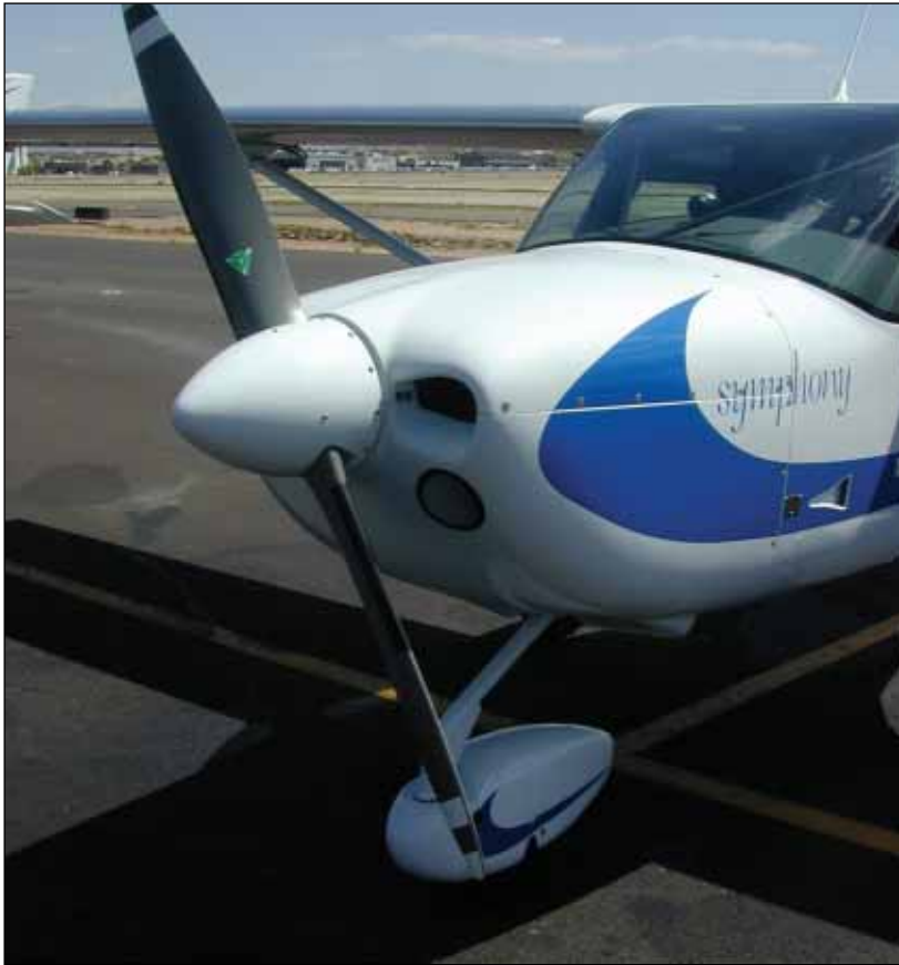
Though the Symphony's propeller may look metal, it's actually a composite MT fixed-pitch in front of the 160-hp Lycoming.
