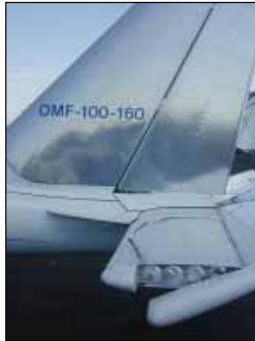
Both the GlaStar (above) and Symphony (at left) feature a composite fuselage shell, but the vertical fin is aluminum on the Symphony and composite on the GlaStar. Piper on the GlaStar's tail refers to the builder's daughter, not the make of aircraft.
