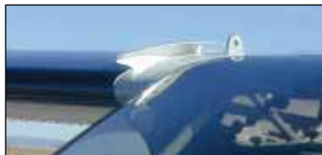
On the GlaStar (left), the vortex generator (VG) is installed at the wingroot. Certification of the Symphony required that the VG move to the inboard end of the aileron.
