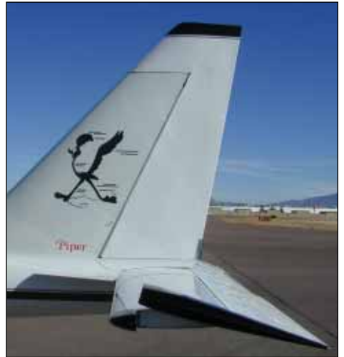
Both the GlaStar (above) and Symphony (at left) feature a composite fuselage shell, but the vertical fin is aluminum on the Symphony and composite on the GlaStar. Piper on the GlaStar's tail refers to the builder's daughter, not the make of aircraft.
