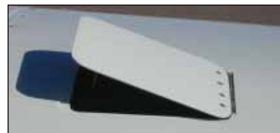
The GlaStar's oil door opens with a vernier control from inside the cockpit. It can help cool the engine after shutdown, or it can be opened in flight.
