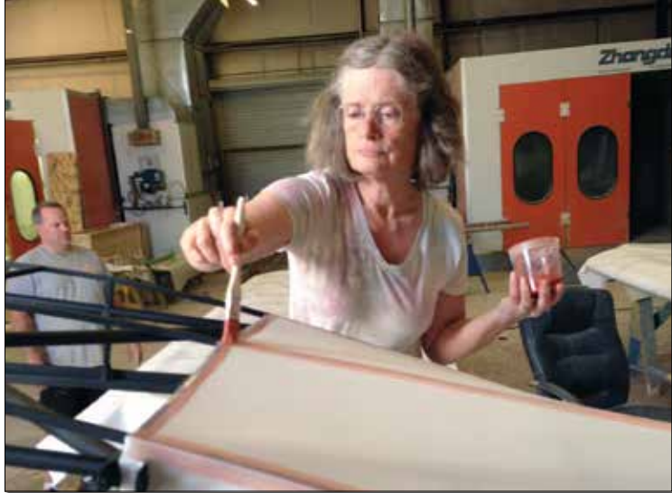
Joan adds glue along all taped joints.
