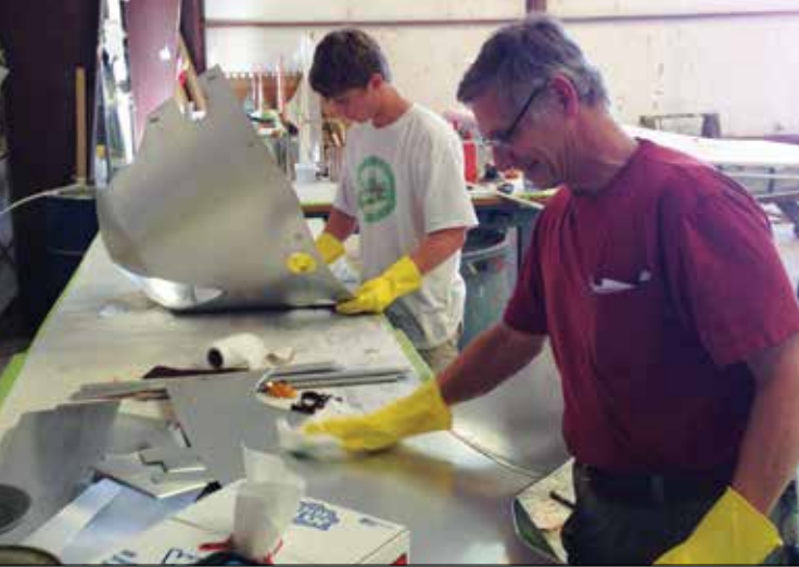
John Paul and father (John) prep and fit the aluminum cowling prior to paint.
